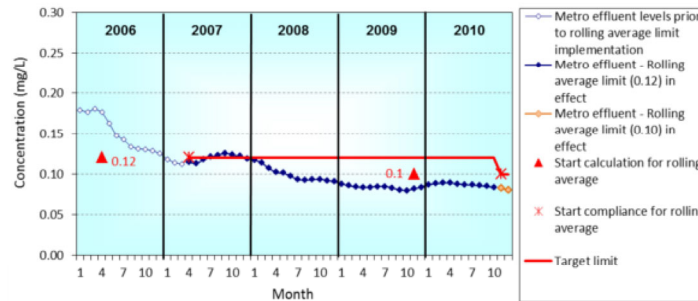
Figure 4-5. Metro TP, 2010 effluent concentration compared to permit limit.
