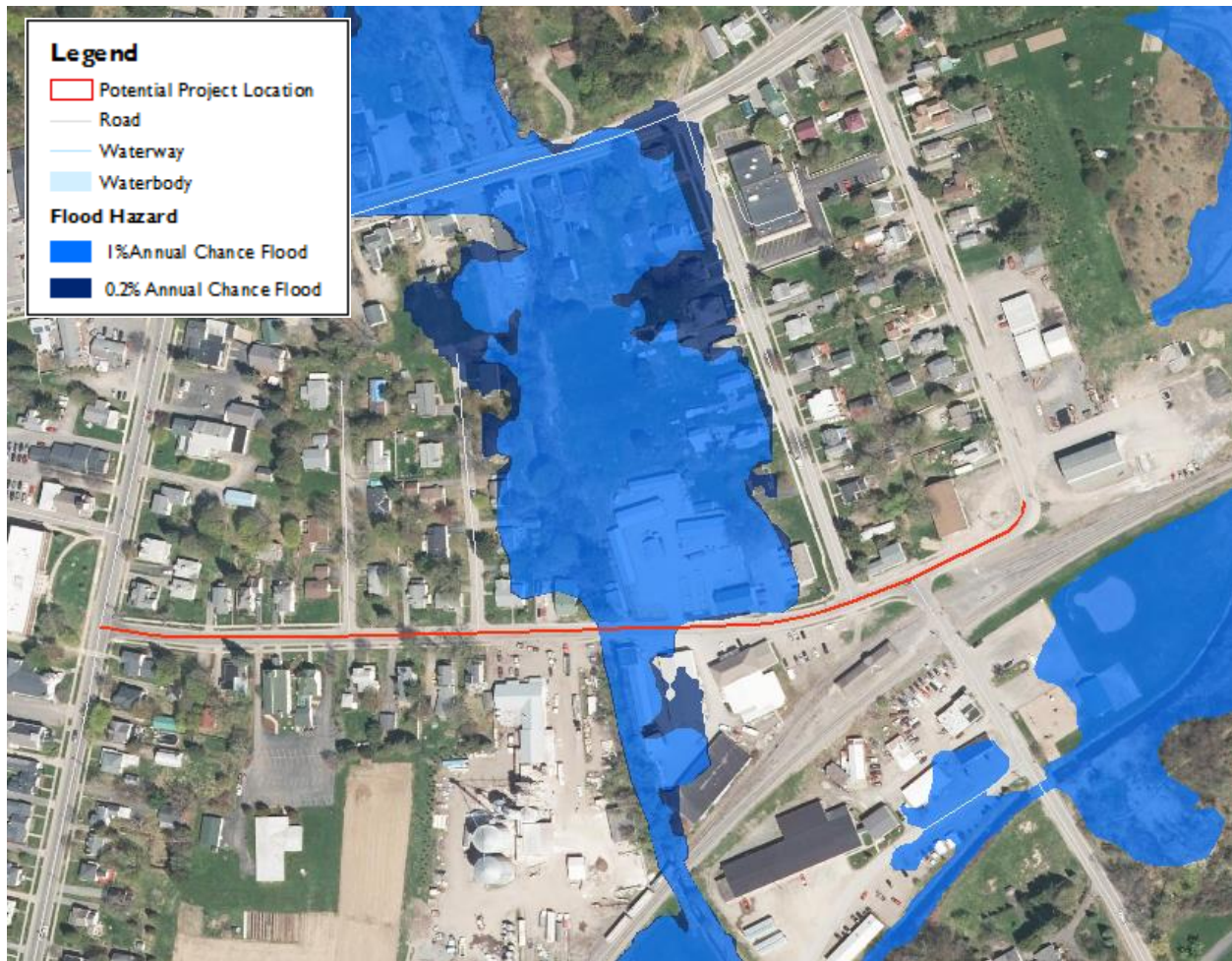
Figure 9.35-4. The map below shows Onondaga Street and Douglas Street near the village highway garage which are prone to flooding due to poor drainage systems.
