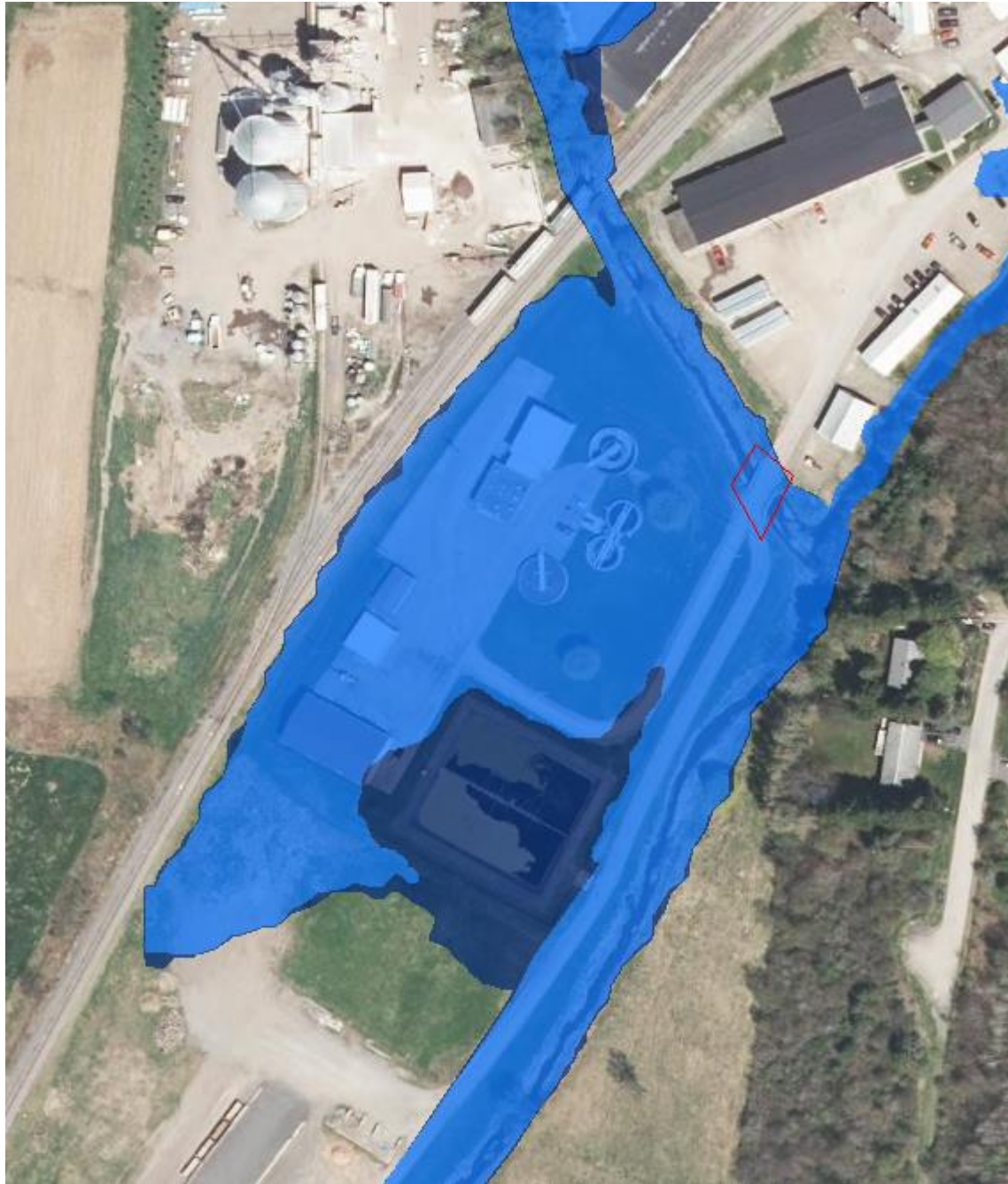
Figure 9.35-3. The FEMA Floodplain was added to the map to highlight the risk that the water treatment plant is in and that the culvert being too small can cause major flooding issue.
