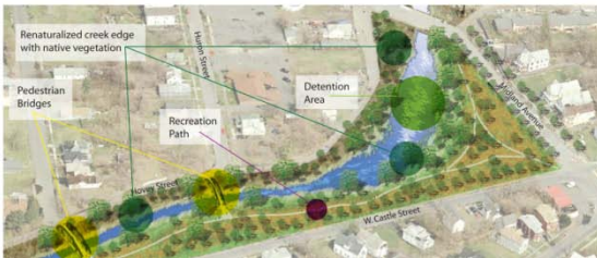
Figure 5.7 Southside preferred project bundle aerial rendering depicting pedestrian bridges over the creek, creekwalk extension, renaturalization, detention area, and new plantings, a cross-section rendering is illustrated above.
