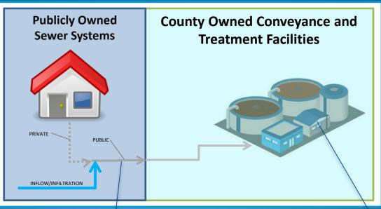
Broken local sewer assets allow inflow & infiltration into the sewer collection system
