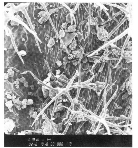
Figure 5-3. Scanning electron microscope micrograph of the adaxial surface of an 8-week-old London plane leaf. Spore, pollen, carbonaceous, angular, and aggregate particles are visible. Scale, 10 \mu m.
