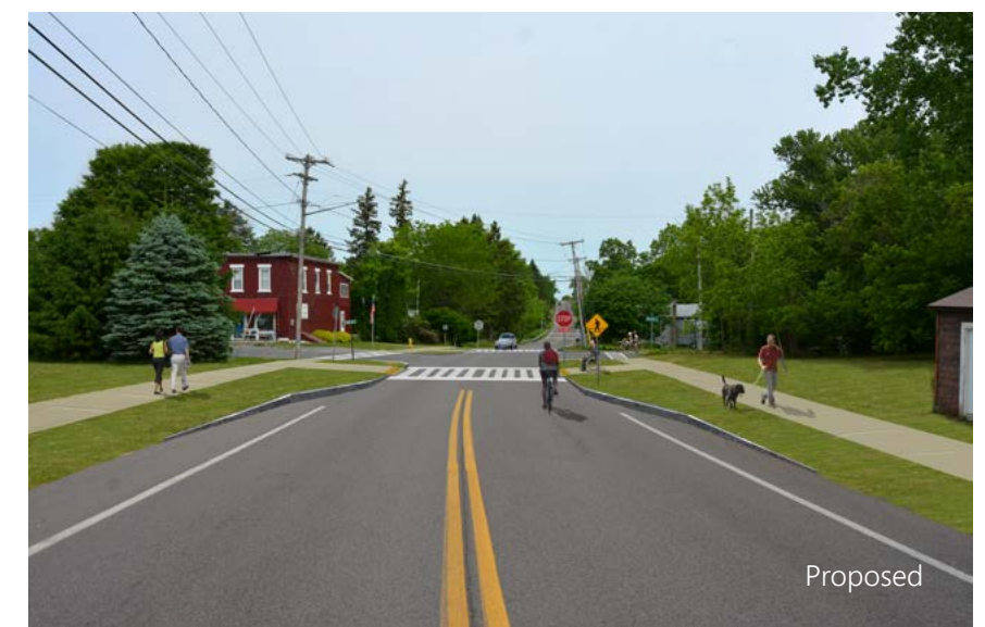
Jordan Road with added sidewalks, bump outs, and crosswalks at the intersection with Mottville Road
