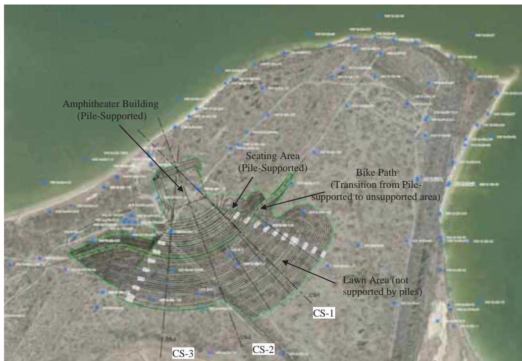
Figure 1. Conceptual Grading Plan and Approximate Locations of Available Soil Borings
